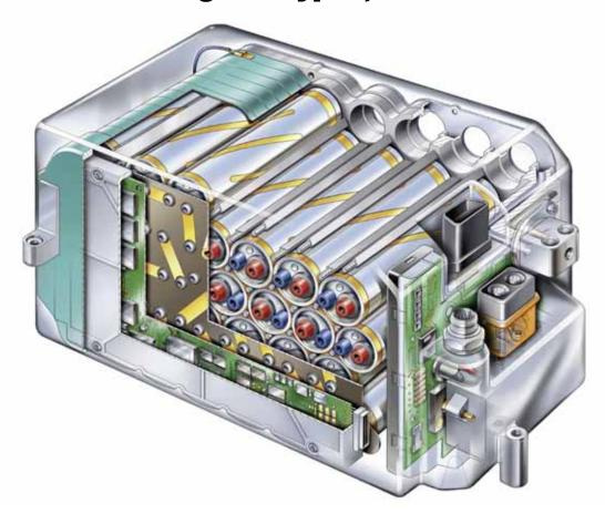
Mercedes-Benz's \$400 Hybrid features a small lithium-ion battery pack comprised of 32 nickelcobalt-aluminum cells manufactured by Saft. The 120-V, 0.9 A-h aircooled pack is assembled by Continental.
